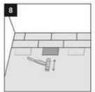
pieces and a small hammer or rubber mallet to gently tap the planks into the click of the previous who was sure they are tightly clicked together and make sure there is no gap between the long ide of the planks installed. ANY GAPPING CAN COMPROMISE THE WHOLE INSTALLATION
