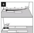
Start the second row with the leftover cut part of the last plank of the previous row. This small plank should measure at least 12'.
