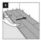
After 2-3 rows. Adjust the distance to the front wall by leaving an expansion gap of 14".
