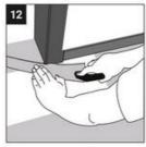
Door molding and skirting: lay a board (with the decorative side down) next to the door molding and as shown in the figure Then slide the floorboard under the mold ing.
