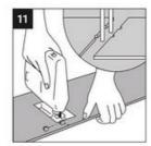
Holes for pipes: measure the diameter of the pipe and drill a hole that is %' larger. Saw off a piece as shown in the figure and lay the board in place on the floor. Then lay the sawed-off piece in place.
