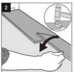
Second plank, first row. Drop the plank and gently press down the end with a rubber mallet so it firmly locks into the previ-ous plank until both planks are at the same height. Make sure both planks are perfectly aligned.
