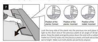
NOTE: If you notice both planks aren't at the same height or are not well locked together please follow disassembling instructions at the end of installation steps; disassemble and check if any debris stuck inside the lock is obstructing.
