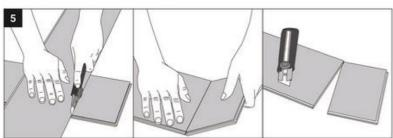
To cut the plank, use a simple utility knife and ruler, and with the top side facing up, cut heavily and several times on the same axis. The knife will not go through the surface but make a deep cut. You can then lift one half of the plank using your other hand to hold down the second placing it very close to the cut. The plank will split naturally.
